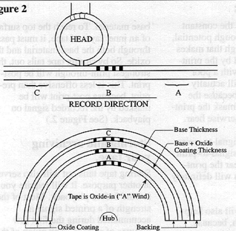
Tape stored on take-up reel. Section C receives most signal transfer, which appears as post-print on playback. This method of storage is recommended for master tapes.
