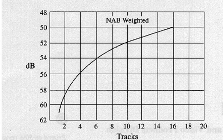
Stray magnetic fields will also increase print-through by several dB. This is one more reason why you should be sure tape heads and guides aren't magnetized. Also no symmetrical bias waveforms (those which produce even order harmonics) can be the cause of problems. These problems will leave DC magnetic fields on the tape and greatly increase print-through. The DC field in effect helps "bias" the oxide to enhance the print-through effect.
